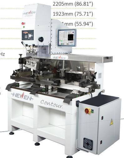
FIXED-TURNING® numerically controlled axes driven by satellite roller screws and servo- motors of the latest generation. A precision of the tool travelling by interpolation is measured in thousandths of mm.
