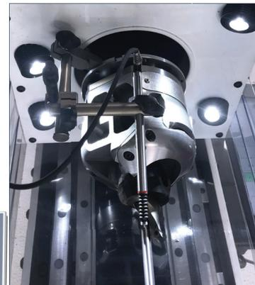
Built-in low-voltage multipoint lighting (LEDs) -- cold light. The work area is particularly well lit, the control of the finished work is improved and, consequently, the operator's fatigue is reduced.
