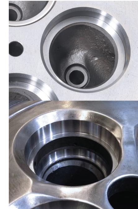
Machining of Venturis to accelerate the speed of gases.
