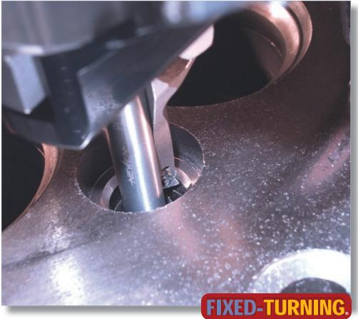
the new standard in valve seat machining<sup>™</sup>
