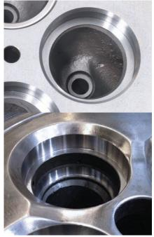
Machining of Venturis to accelerate the speed
