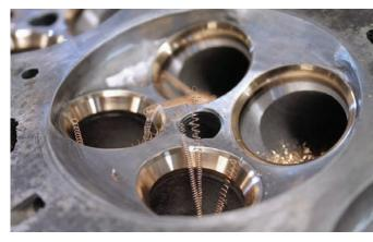
Motorcycle cylinder heads, the smallest valve seats around and to come (downsizing, at the heart of all the new engine development programs) can be machined with utmost ease and the optimum precision of competition engines...
