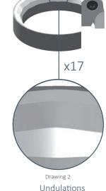
The lapping of powder metal valve seats, or of some cast iron valve seats, brings about unavoidable chatter marks. Chatter marks are very harmful to a valve since gases escape through them while the valve is shut.
