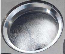
Valve Seat Hardness: 56/58HRC (573HB+ / 610HV50+)
