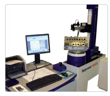
This machine whose resolution is 1/100 of a micron allows to automatically control all geometric parameters that define the quality of a guide and of a valve seat: circularity, concentricity, runout, cylindricity, segment linearity, angle, surface finish... The control reports and graphs resulting from the tests are indisputably recognized by the control departments of the most prestigious OEMs.
